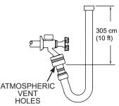
2. Maintain the hose at a height of 305-cm (10 feet) for five minutes while watching the atmospheric vents for leakage.\*
