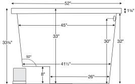
IMPORTANT: Air baths and tubs with a pre-leveled foam base or frame system add 2-3" to overall tub height.
