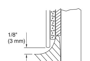
**13 Apply 100% silicone sealant around the shower base where it contacts the finished walls.**
