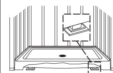
**9 Clean the shower base and cover with a drop cloth. Connect the drain pipe.**
