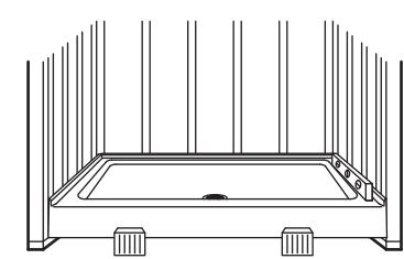
**6 Push down on the front of the shower base.** The installation blocks will be cut and the shower base will rest flat on the floor.
