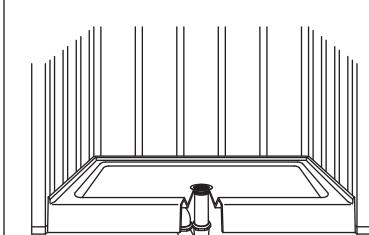
**10 Use furring strips to make the framing flush with the flanges.**
