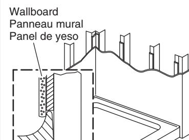
**12 Install the finished wall to within 1/8" (3 mm) of the rim.**
