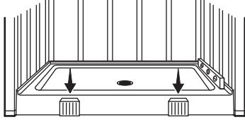
**7 Discard the exterior cut-off blocks.** Verify that the shower base is level and fully supported by the subfloor.
