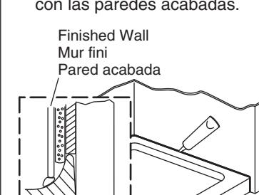
**14** Install the finished floor. Apply 100% silicone sealant along the floor seam.
